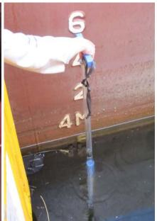
It is recommend to carry out a second draft measurement (after the inclining test/lightweight survey) to verify the data again.
